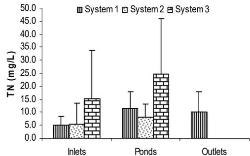
**Fig. 3: TN concentrations (mg/L) in the inlets, culture ponds and outlets of three study systems**
